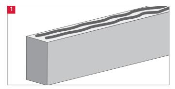
Apply two parallel beads of EGGER Joint & Joist Adhesive to the top of the joist along the first row of boards.
